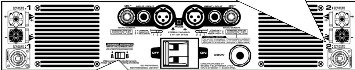
**Floating ground and Transient Suppressor:** Your amplifier circuit ground is insulated from the frame. This allows various safety configurations to be made for the system grounding. For more information, refer to the chapter 6.1 about the Transient Suppressor bar and problems related to lightning systems.
