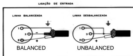
The **X SERIES** amplifiers contain balanced inputs and can be powered either by balanced lines or not, according to the figures.
