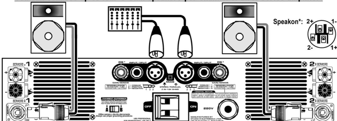
\* Always connect the speaker positive (+) to speakon's pin 1+ or 2+ and the negative to pin 1- or 2- (internally, both pins 1+ and 2+ are connected in parallel. Pins 1- and 2- are also internally in parallel).
