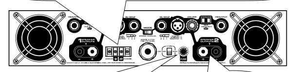
WHEN WE SELECT THE LINE VOLTAGE ON WHICH THE AMPLIFIER WILL OPERATE, IT IS VITAL TO PLACE THE FUSE WITH THE PROPER CURRENT VALUE. SEE THE CORRECT VALUE ON THE FUSES TABLE.
