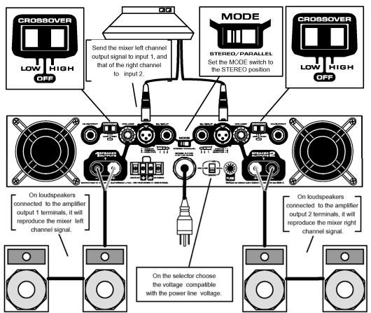
You can connect up to two 8 Ohm speakers or cabinets in parallel per channel, or only one 4 Ohm speaker or cabinet per channel. If you don't respect these limits, you can overload your amplifier and void the warranty.
