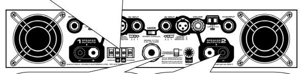
Floating ground and Transient Supressor: Your amplifier circuit ground is insulated from the frame. This allows various safety configurations to be made for the system grounding. For more information, refer to the **chapter 6.1** about the Transient Supressor bar and problems related to lightning systems.
